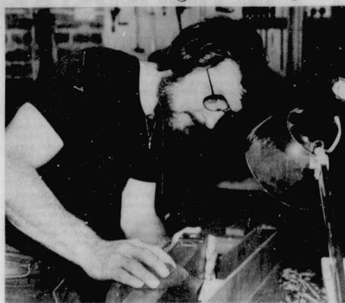
Knud Smenge buffs a wooden Gedackt pipe, made of myrtle and blackwood.
